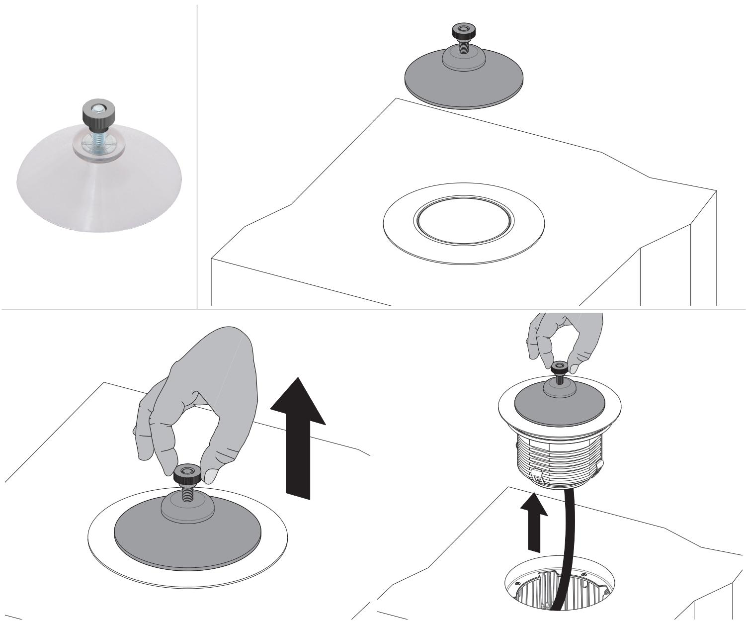
We would like to highlight that such tool is specifically designed to remove the lighting fixtures from their own outer casings. Its successful function can be guaranteed only upon immediate use after installation. Long term installation of the spots is subject to dust and dirt infiltration between the glass frame of the lighting fixture and edges of the outer casing, which works as a binding element. In this case the use of the suction cup would not be enough efficient to perform the removal.
